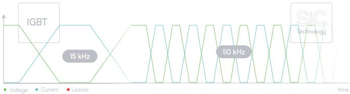
Transitioning to SiC technology results in an increased switching frequency of the converter, which translates into higher dynamics, faster transients and enhanced performance, making it the perfect candidate for EoL environments, R+D, Validation and Power Hardware in The Loop (PHiL) testing.
