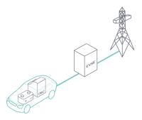
Electric Vehicle Supply Equipment is designed to charge the battery of EV in AC or DC. In AC applications the On Board Charger converts AC in DC.
